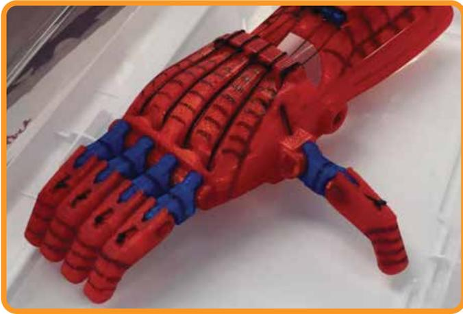
Made nearly entirely of 3D printed parts, the prosthetic operates without a motor. Adduction and abduction of Izzy’s elbow activates two connected, string-like filaments that create movement in her fingers.
